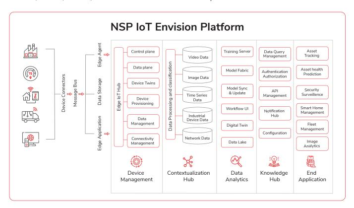
Device Management: The device management is part of Central components. It manages the IoT Edge Gateway and its application remotely. The key features of Device Management components are Edge Gateway provisioning, Remote Application deployment, Remote Application configuration, Remote development of AI/ML components, Dashboard, Notification and reporting services deployment.
